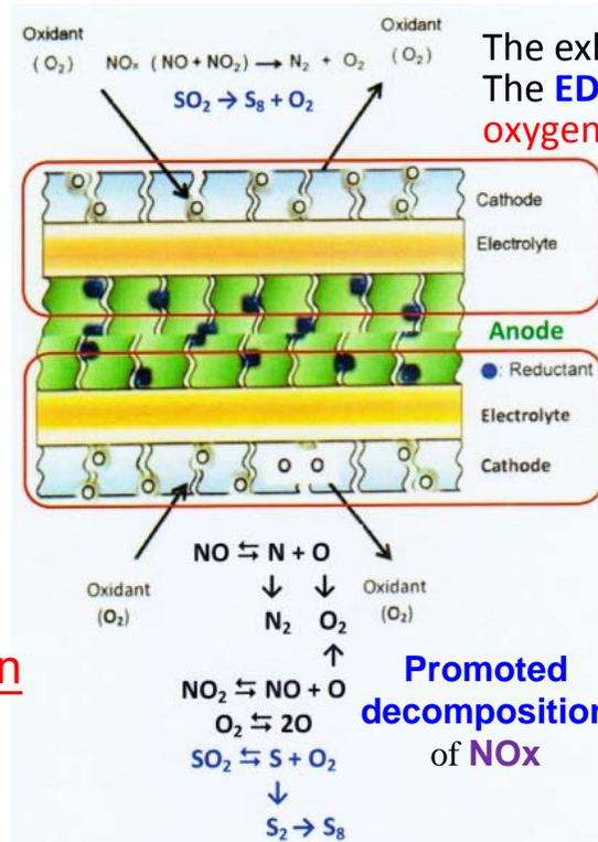
The exhaust flows over the cathode. The **EDC** can **deNO<sub>x</sub>**, needing **facile oxygen desorption**.
