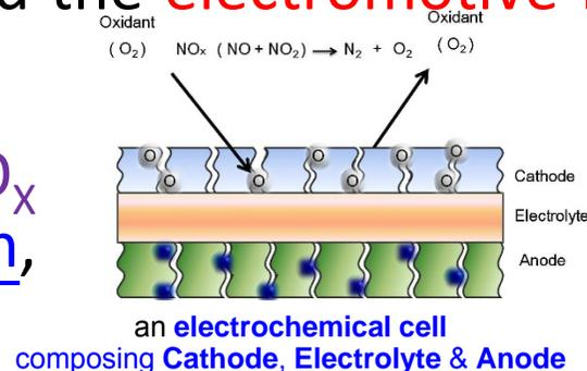
The mobile oxygen ( $O^-$ ) over the cathode surface can promote the oxidation of hydrocarbons (HCs) to result in complete oxidation of HCs
