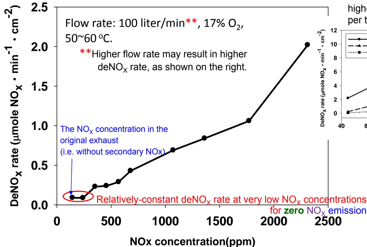
Can be more than 10 times higher than SCR-deNO<sub>x</sub> per treatment area.
