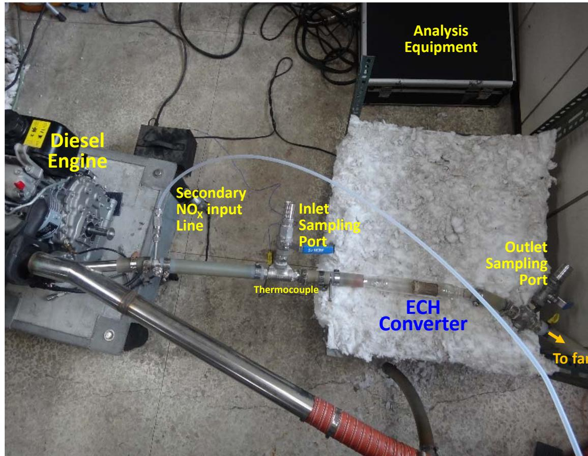
**No reagent or other resource was consumed** in **ECH-deNO<sub>x</sub>**, because the **ECH** converter is simply placed in the exhaust pipe—there is no supply of any reagent or other resource.
